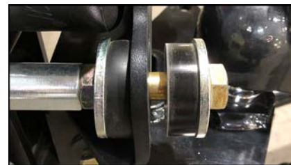
Figure 13: Hitch frame resting on bump cushions closer to tailgate - add air.
