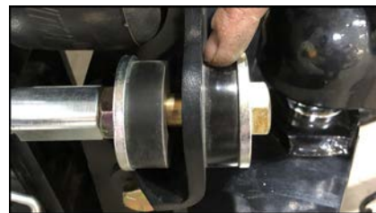
Figure 14: Light trailer-side contact. Stop adding air. Do not compress. Truck-side washers must be free.
