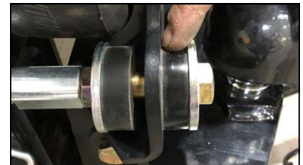
Figure 16: Light trailer-side contact. Stop adding air. Do not compress. Truck-side washers must be free.
