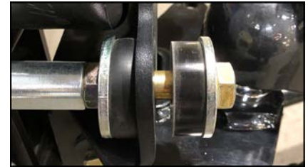
Figure 15: Hitch frame resting on bump cushions closer to tailgate - add air.
