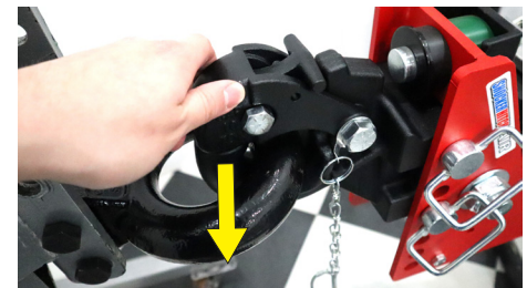
Figure 3: Drop trailer with pintle ring onto pintle hook and push latch down firmly
