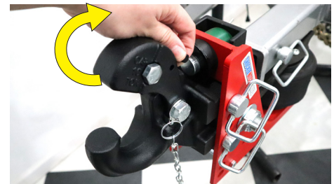
Figure 2: Pull up on latch to open pintle hook
