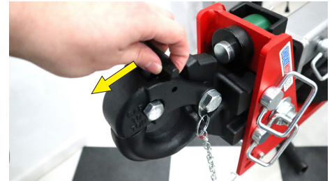
Figure 1: Pull on lever to release latch
