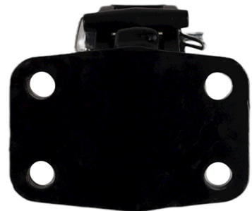
Figure 5: Bolt Pattern on Pintle 1.75" x 3.375 (center to center)
