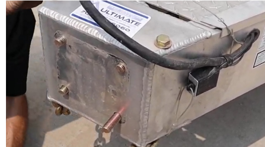
Figure 8: Bolts inserted through inside of trailer
