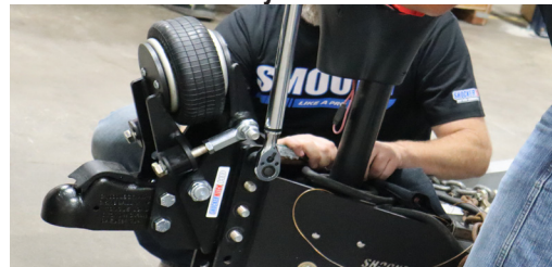
Figure 5: Torque Vertical Channel bolts to 100 ft-lbs
