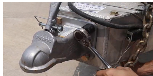
Figure 7: Remove existing coupler
