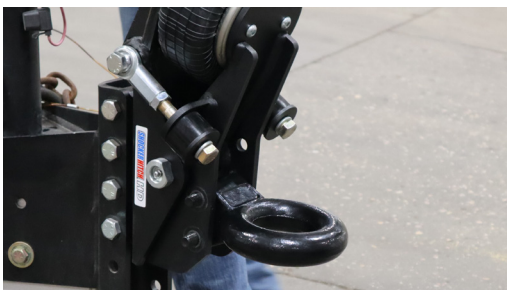
Figure 11: Bolt on Pintle pinned in place
