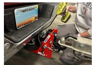
Add air after connecting and loading the trailer.
