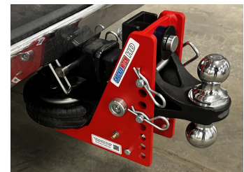
Attachment secured with both pins and retaining clips.
