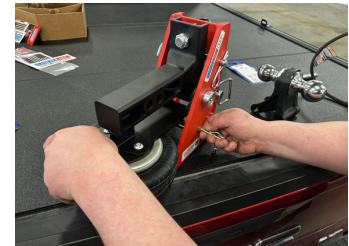
Release air and compress the bag before insertion.
