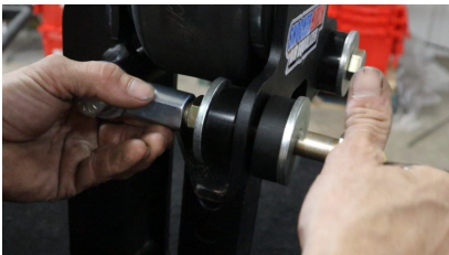
Figure 4: Start screwing in bump cushion assembly bolt until the bolt head is resting on front washer
