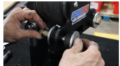
Figure 3: Re-insert bump cushion assembly in correct order
