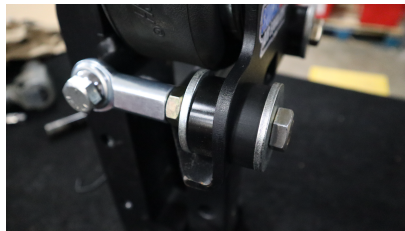
Figure 5: Decompress air bag until the main frame is just touching the front bump cushion
