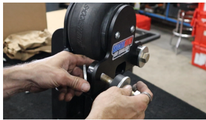
Figure 2: Remove bump cushion assembly from heim
