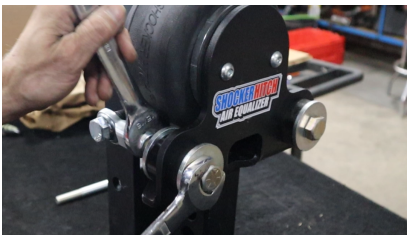
Figure 1: Loosen jamnut on bump cushion bolt
