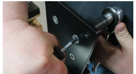
Figure 2: Tighten plated sway ball using a phillips screwdriver & 9/16" wrench.
