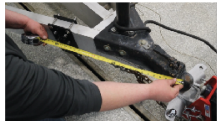
Figure 5: Measure 24" center-to-center from trailer coupler to plated sway ball. For clamp-bolt torque, follow the frame-height conditions in the installation text.
