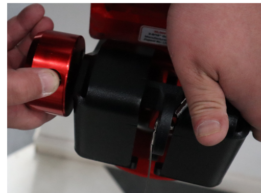
Figure 6: Install Lock onto the protruding end of the Locking Pin
