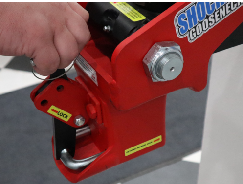
Figure 1: Shift Lock Handle pushed to the unlocked position
