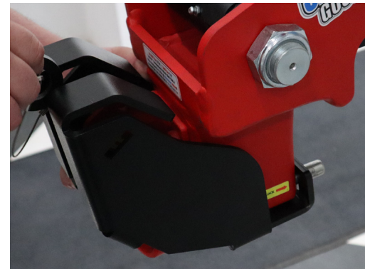
Figure 3: Shift Lock Handle pulled into the locked position
