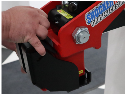
Figure 2: Gooseneck Coupler Lock placed into position
