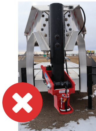
Figure 3: Hitch is crooked: readjust at stem &/or trailer pin
