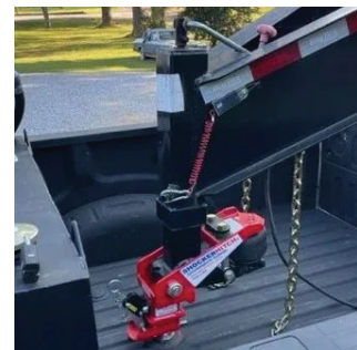
Figure 6: Top crank Gooseneck hitch installed on trailer
