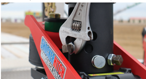
Figure 10: Tighten bolt set bolts snug. Tighten jam nuts after set bolts are snug
