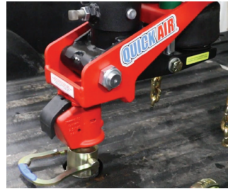
Figure 22: Demco coupler locked onto gooseneck ball
