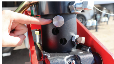
Figure 13: Top hole: For 4" round stems with 10° - 20° angled pin holes
