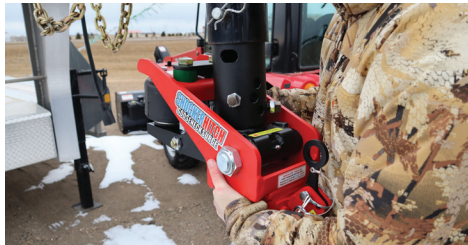
Figure 8: Slide the Standard Frame Gooseneck into Multi-Fit system with air spring bag towards the trailer
