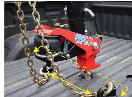
Figure 31: Ideal safety chain location rearward of the ball and 6" to 12" left and right apart from the ball laterally
