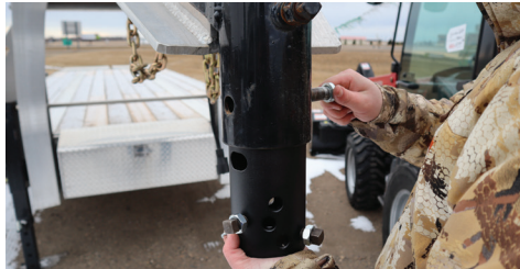
Figure 7: Slide Multi-Fit stem into trailer tube to desired pin hole and secure with 3/4" pin
