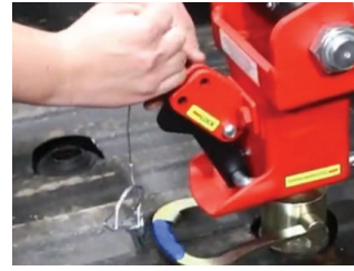
Figure 18: Shift Lock Coupler in correct locked position; 1" of the U-Bolt stick out
