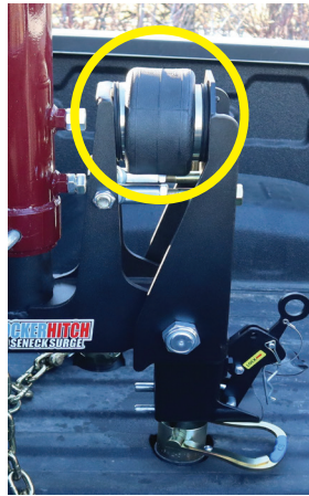
Figure 2: Offset Gooseneck models: air spring bag faces toward the truck cab
