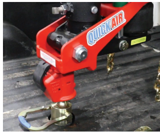
Figure 21: Demco coupler lowered onto gooseneck ball
