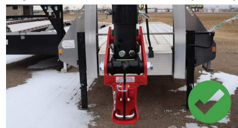
Figure 12: Hitch is straight. No adjustments needed
