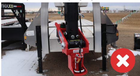
Figure 11: Hitch is crooked. Readjust at universal stem &/or Multi-Fit thru pin
