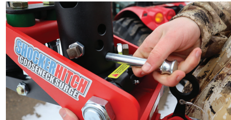
Figure 9: Rotate Standard Gooseneck Frame section until straight with trailer frame and secure with provided pin
