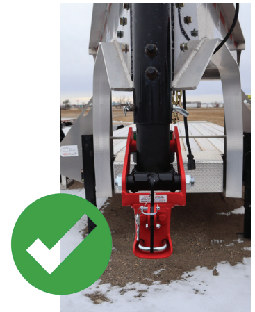
Figure 4: Hitch is straight: no adjustments needed
