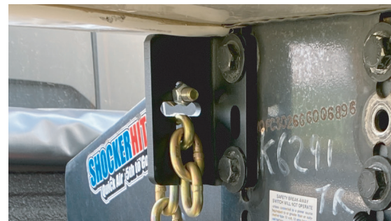
Figure 3: Chain Kit installed correctly (Old Version)
