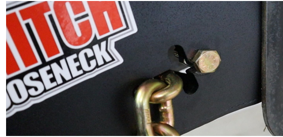
Figure 1: Chain Kit installed correctly (New Version)
