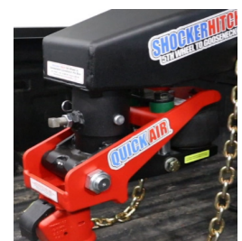
Figure 5: With assistance, insert Quick Air Gooseneck Surge Hitch
