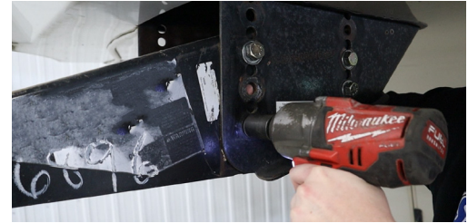
Figure 1: Unbolt existing pin box
