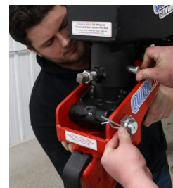
Figure 5: With assistance, insert Quick Air Gooseneck Surge Hitch
