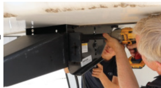
Figure 10: Install safety chain bracket onto pin box frame
