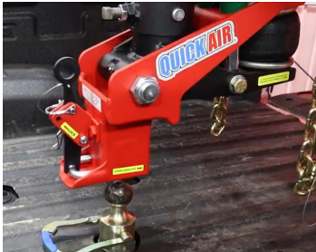
Figure 13: Shift Lock Coupler in unlocked position; lower hitch onto gooseneck ball
