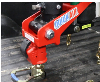
Figure 18: Demco coupler lowered onto gooseneck ball
