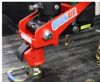
Figure 19: Demco coupler locked onto gooseneck ball
