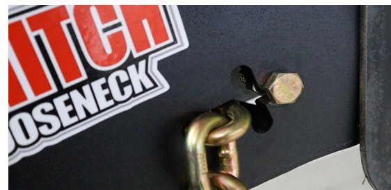
Figure 9: Chain Kit installed correctly (New Version)
