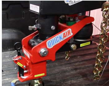
Figure 14: Shift Lock Coupler lowered onto gooseneck ball
