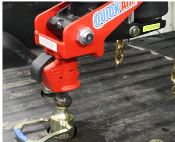
Figure 17: Demco coupler EZ-Latch lowering hitch onto gooseneck ball
