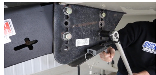
Figure 4: Torque bolts to 120 ft-lbs
