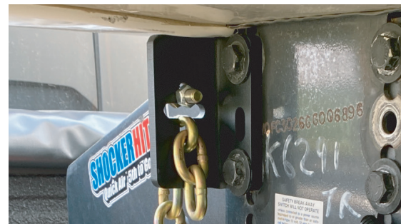
Figure 11: Chain Kit installed correctly (Old Version)
