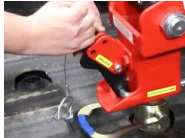
Figure 15: Shift Lock Coupler in correct locked position; 1" of the U-Bolt stick out
