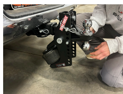
Figure 15: Ball mount installed and secured with hitch pins and clips
