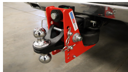
Figure 9: Ball mount installed and secured with hitch pins and cotter pin clips
