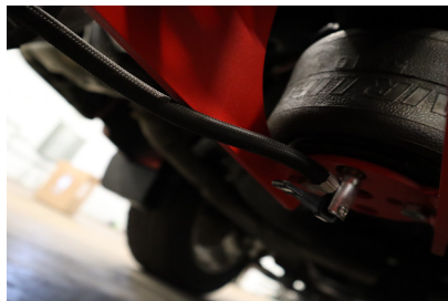
Figure 10: Filling up air spring bag using an air compressor on the valve stem
