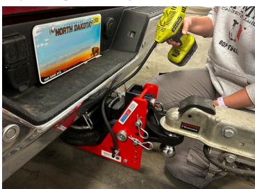
Figure 4: Filling up air spring bag using an air compressor on the valve stem
