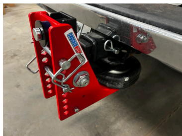
Figure 2: Shank inserted into receiver tube and secured with pin and cotter pin clip
