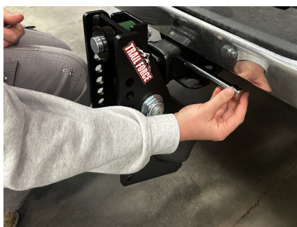
Figure 14: Shank is secured with pin and clip
