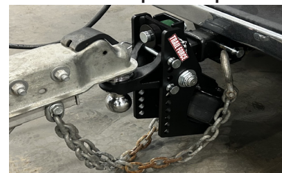
Figure 18: Safety chains and electrical hooked up before towing
