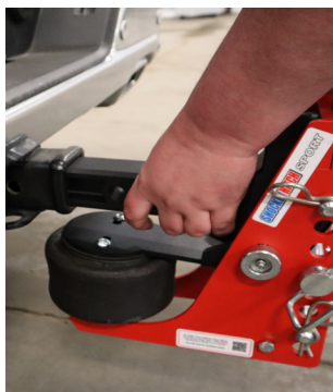
Figure 8: Shank inserted into receiver tube and secured with pin and cotter pin clip
