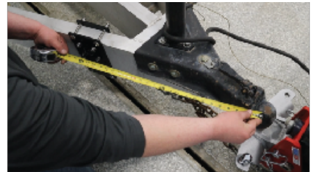
Figure 5: Measure 24" from the center of the trailer coupler to the center of the plated sway ball - tighten down to 24 ft. lbs.
