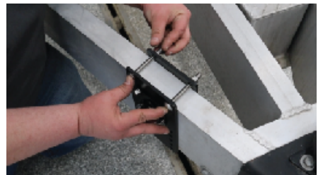
Figure 3: Assemble "back frame" using longer carriage bolts, washers, & nuts on top side.
