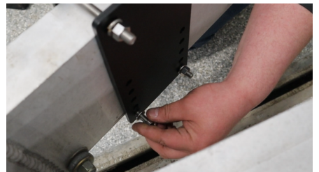
Figure 4: Find desired height and insert the remaining long carriage bolts, washers, & nuts.
