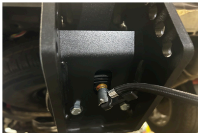
Figure 16: Filling up air bag using an air compressor on the valve stem
