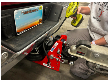
Figure 4: Filling up air bag using an air compressor on the valve stem
