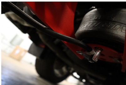
Figure 10: Filling up air bag using an air compressor on the valve stem
