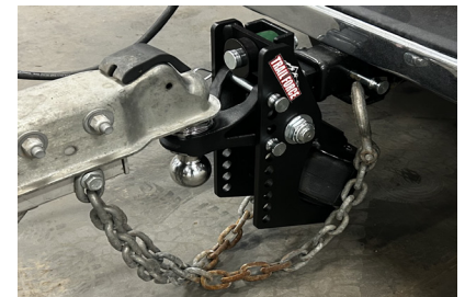
Figure 18: Safety chains and electrical hooked up before towing
