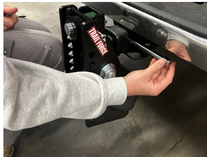
Figure 14: Shank is secured with pin and clip
