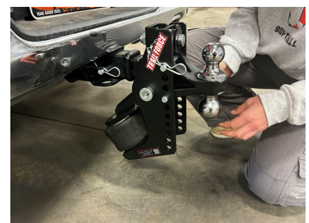
Figure 15: Ball mount installed and secured with hitch pins and clips
