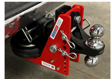
Figure 3: Ball mount installed and secured with hitch pins and cotter pin clips
