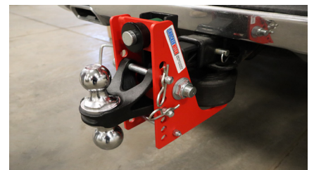
Figure 9: Ball mount installed and secured with hitch pins and cotter pin clips
