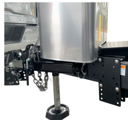
Figure 8: Sway control bars added
