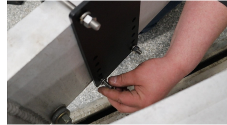
Figure 1: Hand tightening hardware loosely
