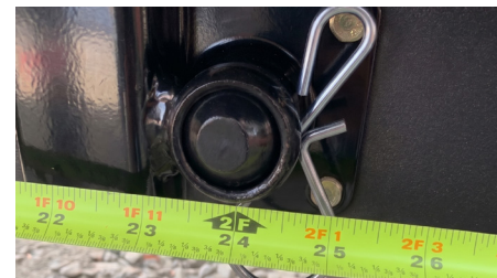
Figure 3: Measurement from center of trailer coupler to center of sway ball is 24"
