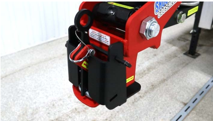
Figure 3: Top insert for 2-5/16" couplers, bottom insert for 3" couplers
