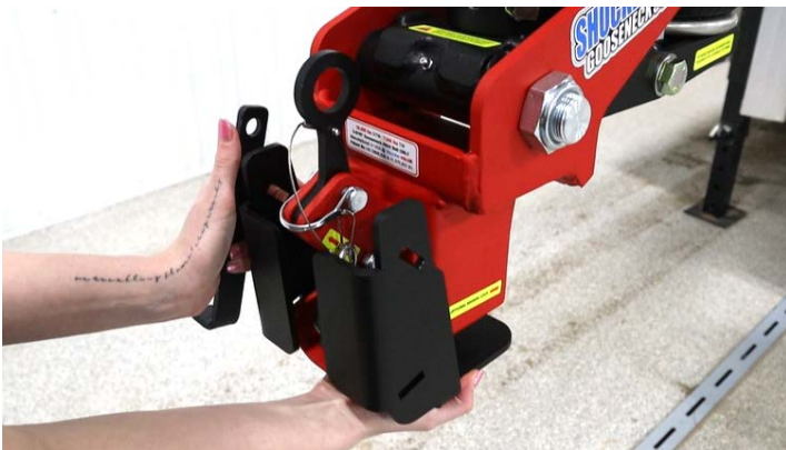
Figure 1: Slide coupler lock frame over Shift Lock®
