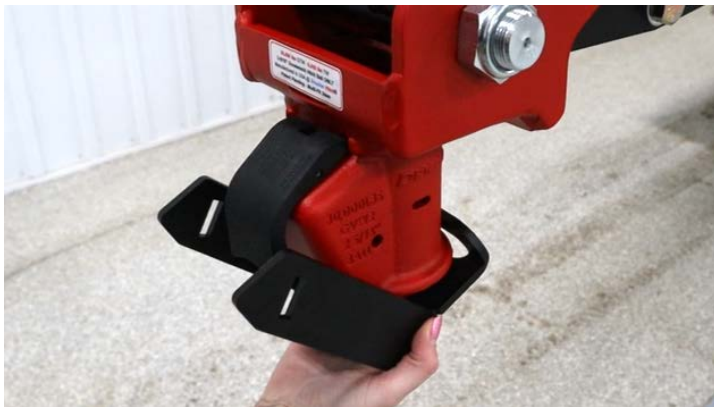
Figure 1: Slide coupler lock frame over Demco coupler
