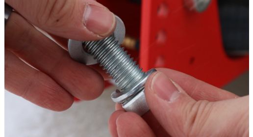
Figure 1: Slide lock washer, regular washer, onto bolt
