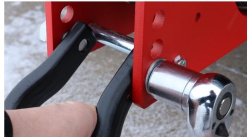
Figure 3: Tighten until lock washer activates - and snug
