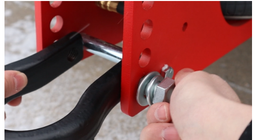
Figure 2: Insert bolt assembly and thread into shackle
