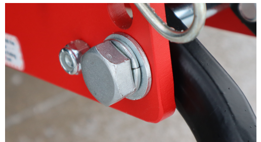
Figure 4: Be sure that lock washer is activated.
