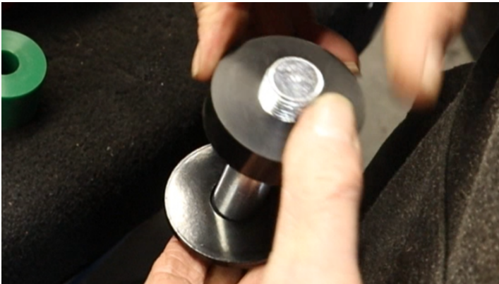
Figure 1: Assemble new top bolt partially, washer than followed by smaller bump cushion.
