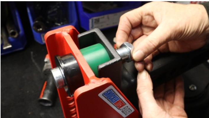
Figure 1: Assemble new top bolt partially, washer than followed by smaller bump cushion.
