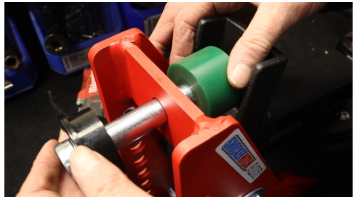
Figure 2: Take bigger bump cushion and insert in between main frame and shank - slide partially assembled kit.
