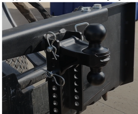
Figure 8: Using (2) 5/8" x 4 1/2" pins, installed desired Shocker ballmount adapter in vertical channel at optimal height
