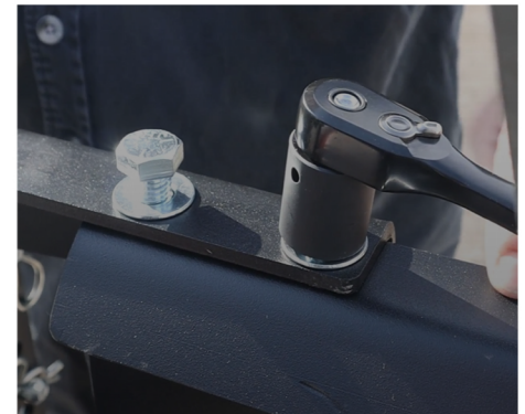
Figure 6: Tighten all hardware progressively until all bolts & nuts are torque to 100 ft lbs
