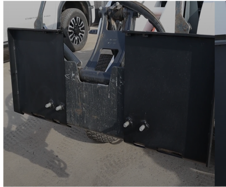
Figure 2: Install both sides of skid steer mounting plate
