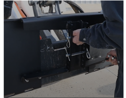
Figure 3: Install center "H" section on side mounting plates
