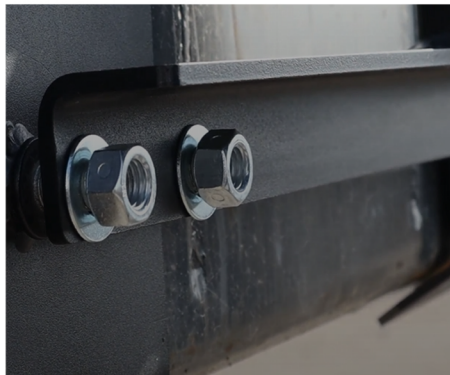
Figure 5: Use (4) 5/8" centerlock nuts & (4) remaining washers on bottom studs. Finger tighten
