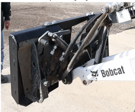
Figure 7: Make sure skid adapter is flush. Engage machine locking levers
