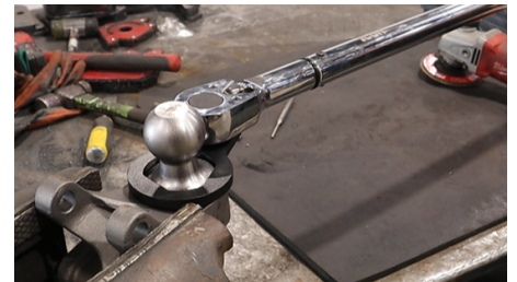
Figure 3: Attach wrench onto 2" side of combo ball and torque to 400 lbs. ft. (repeat if necessary).
