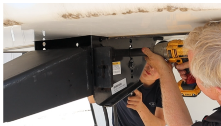
Figure 3: Line up Quick Air® pin box & install with original hardware
