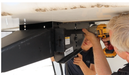
Figure 5: Install safety chain bracket onto pin box frame
