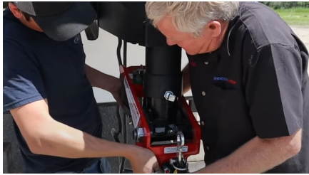
Figure 7: Insert Shocker Hitch into the outer tube of the pin box
