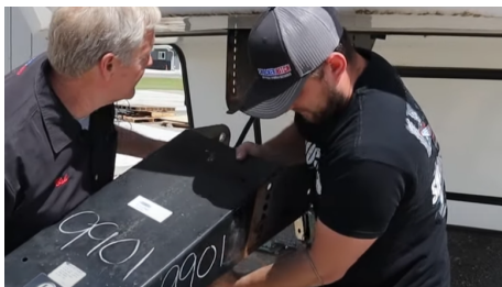
Figure 2: Remove your existing pin box and set aside
