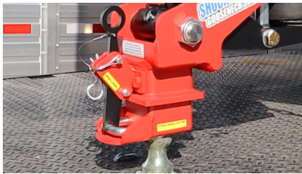
Figure 9: Lower hitch onto gooseneck ball
