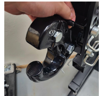
Figure 4: Pulling upward on the lever, open the pintle hook horn.
