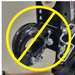
Figure 2: DO NOT install pintle hook "upside down"
