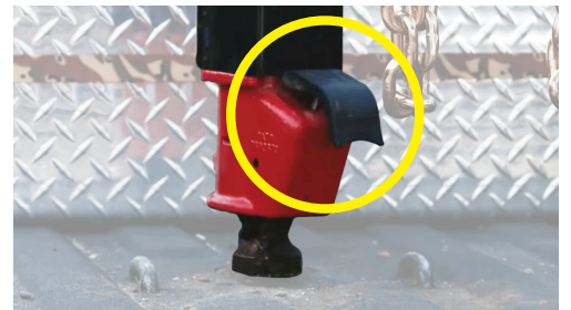
Figure 3: EZ Latch handle starting to lift as trailer is lowered onto ball.
