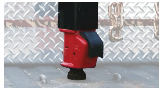
Figure 4: Coupler is fully locked when EZ Latch handle "snaps" back into place.
