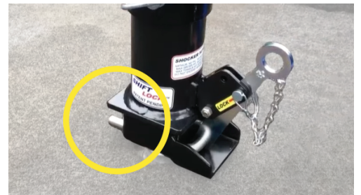
Figure 2: Shift Lock coupler in correct locked position - 1" of u-bolt sticking out.
