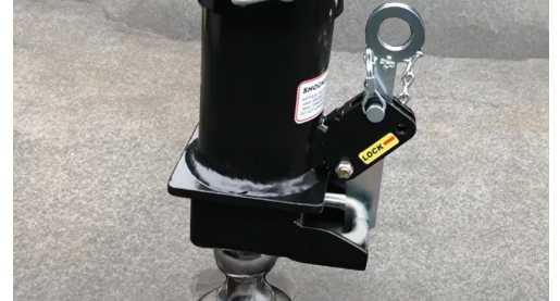
Figure 1: Shift Lock in unlocked position, lower onto gooseneck ball.
