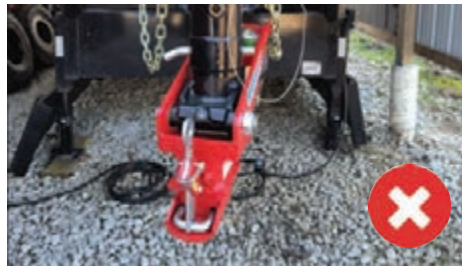
Figure 9: Hitch is crooked. Readjust at universal stem &/or trailer through pin.
