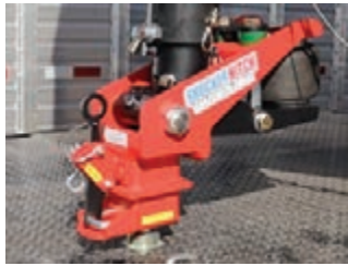
Figure 16: Shift Lock coupler lowered onto gooseneck ball.
