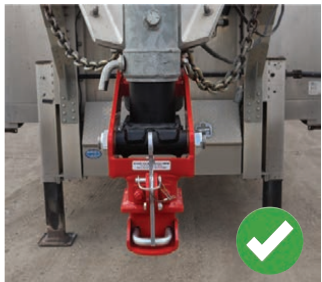
Figure 4: Hitch is straight. No adjustments needed.
