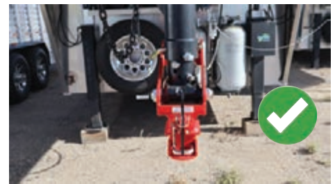
Figure 10: Hitch is straight. No adjustments needed.
