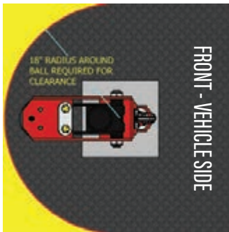
Figure 19: Hitch must rotate at an 18" radius around the ball to prevent contact with items in bed (red frame).
