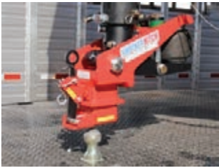
Figure 15: Shift Lock coupler in unlocked position, lower hitch onto gooseneck ball.
