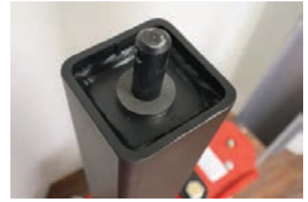
Figure 14: Provided 3/8" washer for top crank goosenecks.
