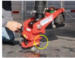
Figure 17: Shift Lock coupler in correct locked position. 1" of the u-bolt stick out.
