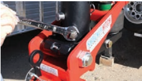
Figure 8: Tighten smaller set-bolt snug. Tighten jam nut.
