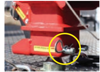
Figure 18: Optional manual lock pin on back of u-bolt (driver's side).
