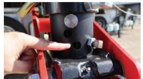
Figure 13: Bottom hole: Round stems with straight pin holes.
