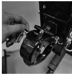
Figure 3: Pull safety pin from pintle hook latch lever
