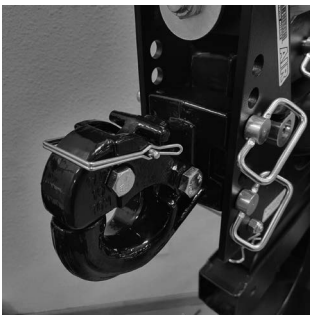
Figure 1: Install pintle hook with the lever facing upward
