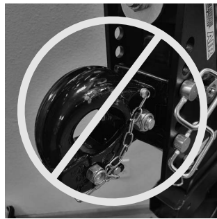
Figure 2: DO NOT install pintle hook "upside down"
