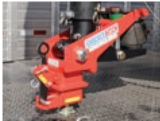
Figure 16: Shift Lock coupler lowered onto gooseneck ball.
