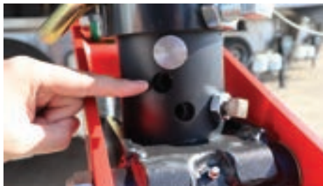
Figure 12: Middle hole: For 100mm round stems with 20°-30° angled pin holes.
