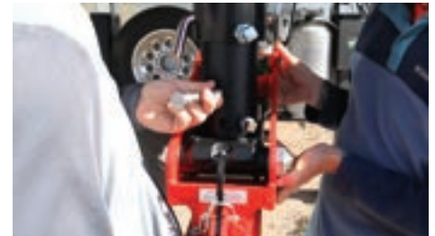
Figure 7: Rotate red frame section until straight with trailer frame and secure with provided pin.
