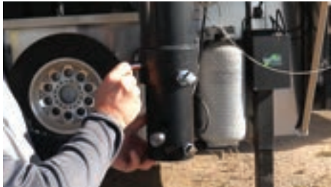
Figure 5: Slide Multi-Fit stem into trailer tube to desired pin hole and secure with 3/4" pin.
