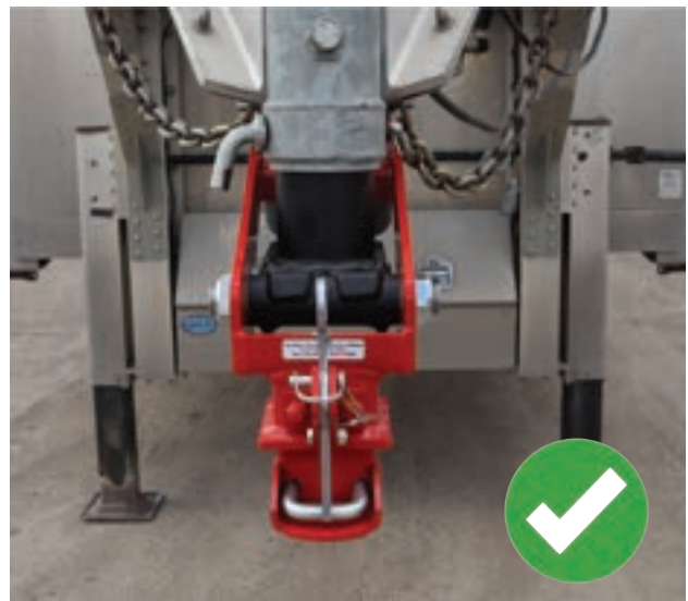
Figure 4: Hitch is straight. No adjustments needed.
