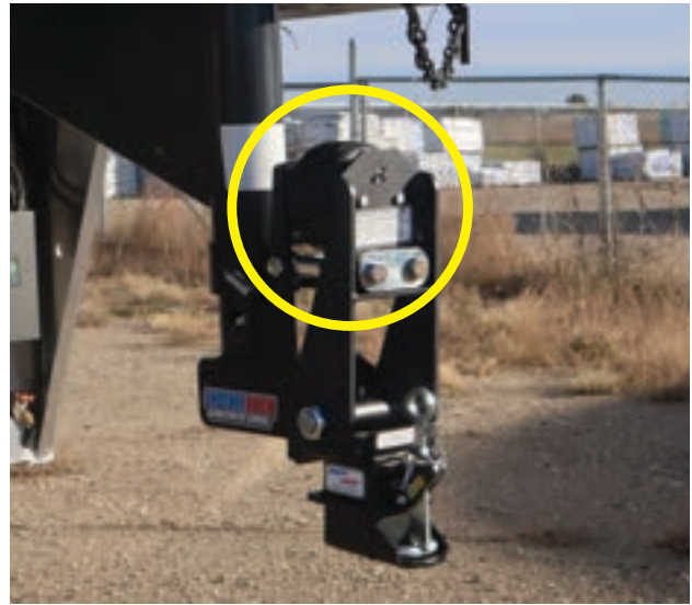
Figure 2: Offset black frame models: Air bag faces toward truck cab.
