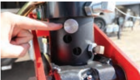
Figure 11: Top hole: For 4" round stems with 10°-20° angled pin holes.
