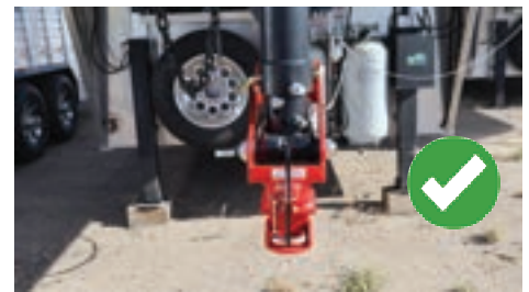
Figure 10: Hitch is straight. No adjustments needed.
