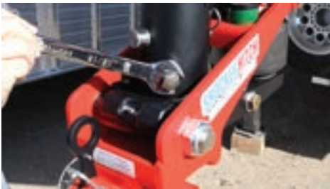
Figure 8: Tighten smaller set-bolt snug. Tighten jam nut.
