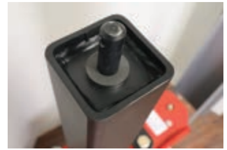
Figure 14: Provided 3/8" washer for top crank goosenecks.
