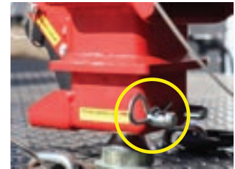
Figure 18: Optional manual lock pin on back of u-bolt (driver's side).
