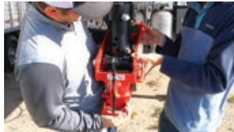
Figure 6: Slide red frame section into Multi-Fit system with air bag toward trailer.
