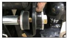
Figure 16: Hitch frame resting on bump cushions closer to trailer - stop adding air.
