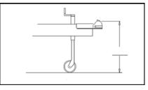
Figure 8: On a level surface, measure the height of your trailer coupler to ground.
