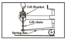
Figure 6: Center the lifting bracket parallel with the spring bar chains.
