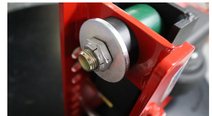
Figure 2: Tighten the jamnut until ONLY 2-3 threads of the top bolt are showing through the jamnut
