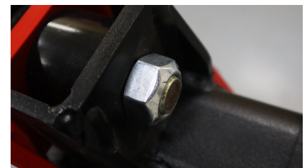
Figure 4: Tighten the top bolt nut until it is showing 1-2 threads past the nut
