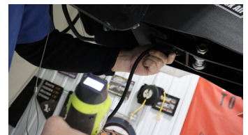
Figure 5: Adjust the air pressure of the Shocker Hitch unit using the air valve located on the bottom side
