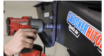
Figure 2: Line up Quick Air pin box and install with original hardware
