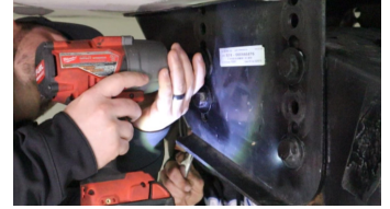
Figure 1: Loosen pin box bolts & nuts and remove original pin box
