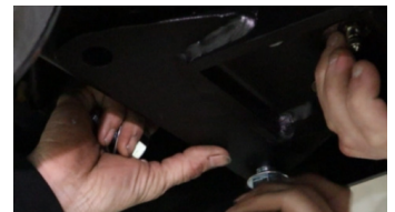
Figure 4: Thread provided bottom side hardware by hand & tighten with impact wrench with 5/8" socket
