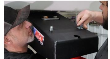
Figure 3: Line up Shocker Hitch unit with pin box & thread provided topside hardware by hand
