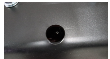
Figure 6: Grease fitting located on the top of the Quick Air pin box once Shocker Hitch is installed
