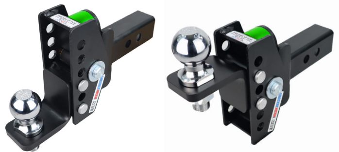
FIGURE 2: GREEN bushings facing "upward" the weight is on the ORANGE bushing - 3,500 lb GTW & 350 lbs TW
