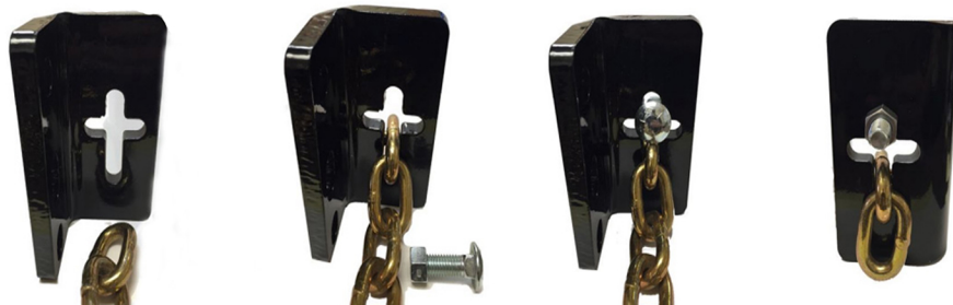
Figure 2, 3, 4, & 5: Slide chain through bracket to desired length and use carriage bolt to hold in place
