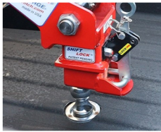
Figure 6: Shift Lock coupler in unlocked position
