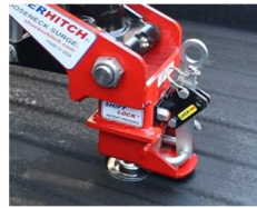
Figure 7: Shift Lock coupler lowered on gooseneck ball
