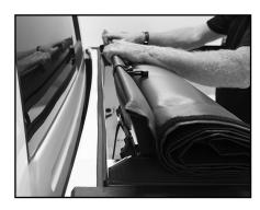
C. Slide left tension adjuster until it engages under side rail (see Step 5F). Push bar back and forth to line up holes. Do not turn adjustment wheel. Insert bolt from top then secure with washer and nut from bottom.
