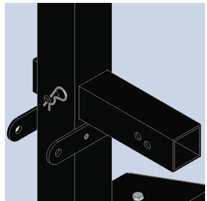
Figure 6: Secure pin with hair pin clip.
