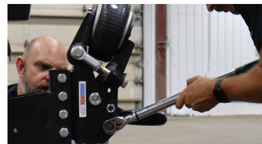
Figure 13: Bolts torqued to 100 ft-lbs
