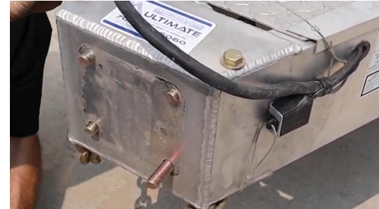
Figure 8: Bolts inserted through inside of trailer
