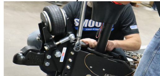
Figure 5: Torque Vertical Channel bolts to 100 ft-lbs
